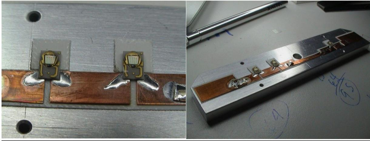
**Figure 2.1.11: Properly Preheated Then Hot Air Penciled Solder Joints**
