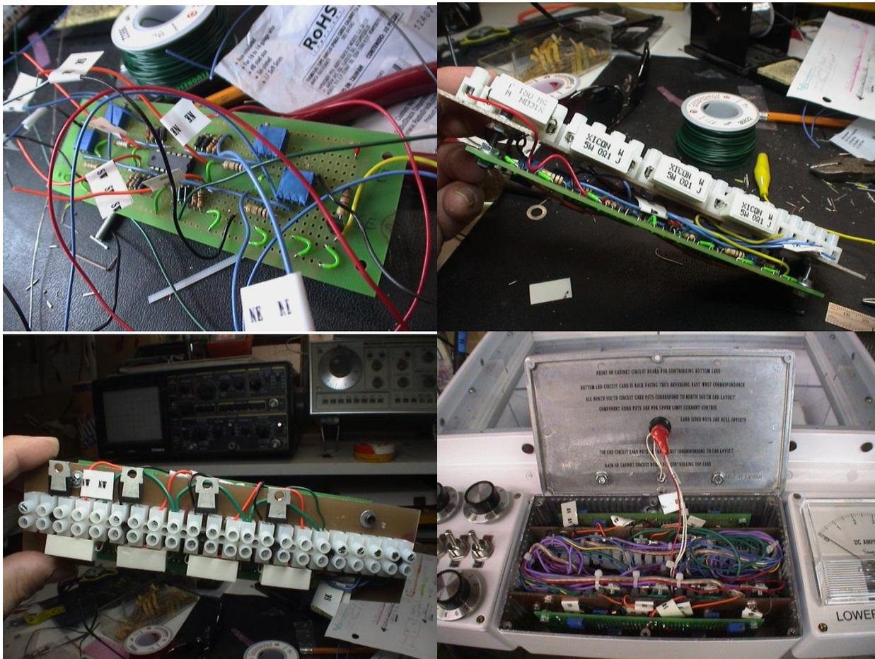
**Figure 2.1.8: Twin Quad LED Driver Circuit Cards**
