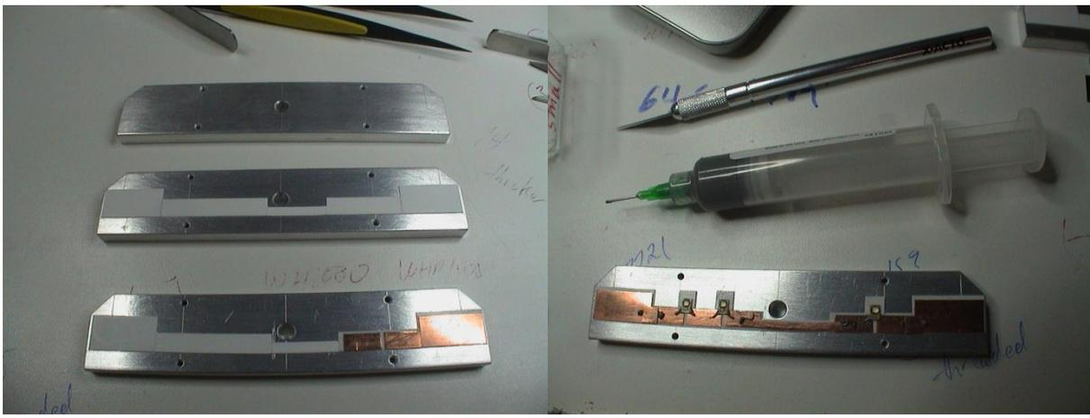
**Figure 2.1.10: Component Placement Ready for Solder Paste to Be Melted**
